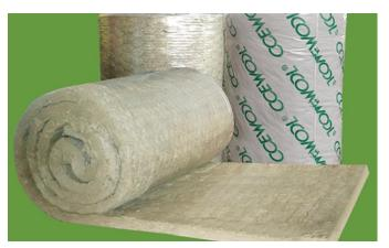
CCEWOOL® Stone Wool Blanket with Wire Mesh is manufactured in rolls, which is made from stone wool felt and galvanized iron wire mesh sewn together with galvanized iron wire. It features good elasticity, thermal preservation, and easy construction. Water repellent type and low chlorine type of products can be manufactured according to
