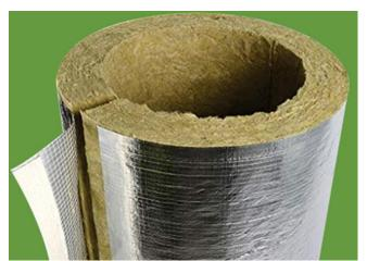
CCEWOOL heat-resistance Stone Wool Pipe is made of stone wool fiber rolled by amold and cured under high temperature. For easy installation, it can be cut along the axis of the shell to facilitate construction. It ensures the tight coupling between the shell and the pipelines that needs insulation. The
