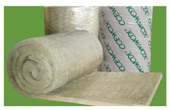
CCEWOOL heat-resistance Stone Wool blanket with Wire Mesh is manufactured in rolls, which is made from stone wool felt and galvanized iron wire mesh or stainless-steel wire mesh sewn together with galvanized iron wire or stainless-steel wire. It features good elasticity, thermal preservation, and easy construction. Water repellent type and low
