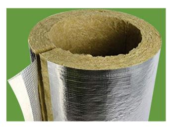
CCEWOOL heat-resistance Stone Wool Pipe is made of stone wool fiber rolled by amold and cured under high temperature. For easy installation, it can be cut along the axis of the shell to facilitate construction. It ensures the tight coupling between the shell and the pipelines that needs insulation. The outer surface of the shell can be polished according to the requirement of customers to achieve the exact
