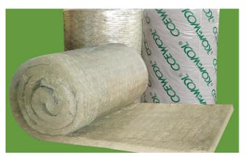
CCEWOOL heat-resistance Rock Wool blanket with Wire Mesh is manufactured in rolls, which is made from Rock wool felt and galvanized iron wire mesh or stainless-steel wire mesh sewn together with galvanized iron wire or stainless-steel wire. It features good elasticity, thermal preservation, and easy construction. Water repellent type and low
