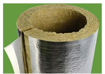
of Rock wool fiber rolled by amold and cured under high temperature. For easy installation, it can be cut along the axis of the shell to facilitate construction. It ensures the tight coupling between the shell and the pipelines that needs insulation. The outer surface of
