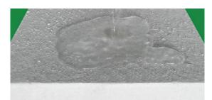
Temperature Grade 1100°C (2012°F), 1260°C (2300°F) CCEWOOL® Water Repellent Ceramic Fiber Board is a kind of refractory ceramic fiber board which combines water proof, thermal insulation and fire resistance in one. We added a hydrophobic formula to the raw materials, and use full automatic production line, 2 hours deep
