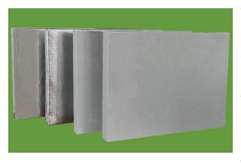
Temperature Grade: 900°C (1652°F) CCEWOOL® M90 Microporous Insulation Board is an efficient insulation product based on advanced microporous insulation technology. It has a lower thermal conductivity than stagnant air, making it an ideal high-temperature insulation material. The surface of the board can be coated with aluminum foil or PE shrink film. The nano board can also be
