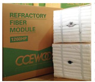
Temperature Grades: 1100°C (2012°F), 1260°C (2300°F), 1400°C (2550°F), 1430°C (2600°F) CCEWOOL® Ceramic Fiber Module is made from spun refractory ceramic fiber blanket, mechanically processed, and produced according to customer drawings. The product is pure white in color, with uniform dimensions, and can be directly fastened to the steel plate anchor pins on the industrial kiln shell, providing excellent fire resistance and insulation, thereby improving the overall
