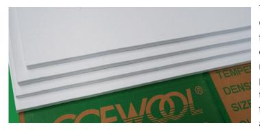
Temperature Grade 1260 °C (2300 °F) CCEWOOL® Ceramic Fiber Board LD is made from high-purity alumina-silicate fibers with a certain proportion of binders added. It is manufactured through processes such as pressing, curing, shaping, longitudinal and transverse cutting, and vacuum molding. It features a uniform structure, excellent thermal and acoustic insulation properties, low thermal
