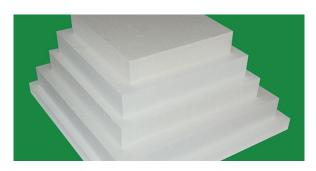
Temperature Grade  $1260\,^{\circ}\mathrm{C}(2300\,^{\circ}\mathrm{F})$  CCEWOOL® Ceramic Fiber Board HD insulation material is a high-density board product made primarily from alumina-silicate fibers with the addition of binders. This product has a tough texture, excellent self-supporting strength, and compressive strength, making it highly resistant to the impact of molten metals. The compressive
