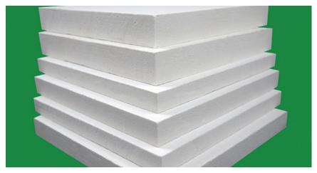
Temperature Grade **1260℃(2300**℉) CCEWOOL® Ceramic Fiber Board RG insulation material is an economical and efficient insulation board. The surface of the board is coated with a hardening agent, which, after drying, provides the board with rigid characteristics. It is suitable for applications that require rigid strength in the product. This material offers high resistance to
