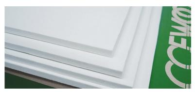
Temperature grade 1300 ℃ (2372 ℉) CCEWOOL® Low Biopersistent Fiber Board 2372 is the latest development in soluble fiber products, made from a blend of soluble fiber cotton, organic, and inorganic binders, forming a hard board. In use, Low Biopersistent Fiber Board maintains high compressive strength and low thermal conductivity,
