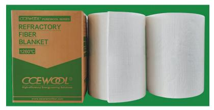
Temperature Grades 1260° C (2300° F) and 1430° C (2600° F) CCEWOOL® PUREWOOL Ceramic Fiber Blanket is a premium product among refractory ceramic fibers. It is made from upgraded materials using high-purity alumina, zirconia, and silica as raw materials. Due to its extremely low impurity content, this blanket is whiter in color. Ultra-long spun fibers are interlocked through a double-sided
