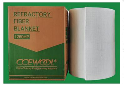
Temperature Grade 1260° C (2300° F) CCEWOOL® Ceramic Fiber Blanket HPS, purified from raw materials with fewer impurities, is made from high-purity refractory ceramic fiber spun fiber. Compared to RCF Blanket S, this product is whiter and has a lower thermal conductivity. It contains no organic binders. Manufactured through a unique internal needle punching process, with tensile strength exceeding 85KPa, providing higher performance and
