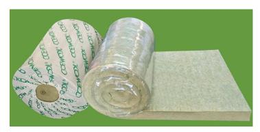
CCEWOOL Rock Wool Blanket is flexible and can well fit irregular equipment and large pipes. Its good length can effectively reduce the number of joints and thermal bridges. Water repellent type and low chlorine type of products can be manufactured according to the
