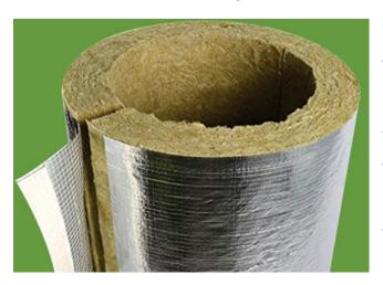
of rock wool fiber rolled by amold and cured under high temperature. For easy installation, it can be cut along the axis of the shell to facilitate construction. It ensures the tight coupling between the shell and the pipelines that needs insulation. The outer surface of the shell can be polished according to the requirement of customers to achieve the exact
