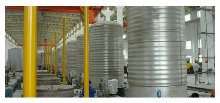
A hood-type furnace is a piece of equipment used for the bright annealing and heat treatment of workpieces. It falls under the category of intermittent variable-temperature furnaces, with operating temperatures typically ranging from 650 to 1100°C, following prescribed heating profiles over time.
