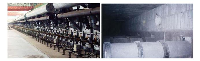
In a CSP (Compact Strip Production) line, the normal furnace temperature is 1220°C. High-speed burners are used, installed alternately on both sides of the furnace wall. Fuels commonly used include gas and natural gas. The operating atmosphere inside the furnace is weakly oxidative.
