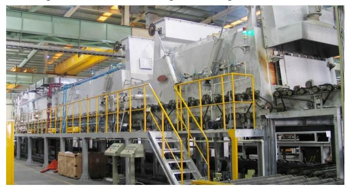
The thin slab continuous casting and rolling process is a compact and efficient furnace technology. It involves taking 40-70mm thick slabs cast by a continuous caster, heating them uniformly or locally, and then sending them directly to a hot strip rolling mill to be rolled into 1.0-2.3mm thick steel strips.
