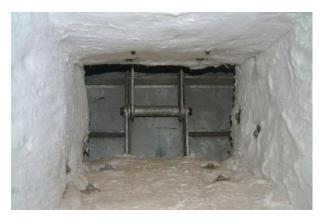
It adopts a layered-module composite lining structure with CCEWOOL 1260 ceramic fiber blankets for the back lining and CCEWOOL1430 zirconium-containing ceramic fiber modules for the hot surface. The ceramic fiber modules are arranged like "a battalion of soldiers", and the interlayer compensation blanket uses CCEWOOL1430 zirconium-containing ceramic fiber
