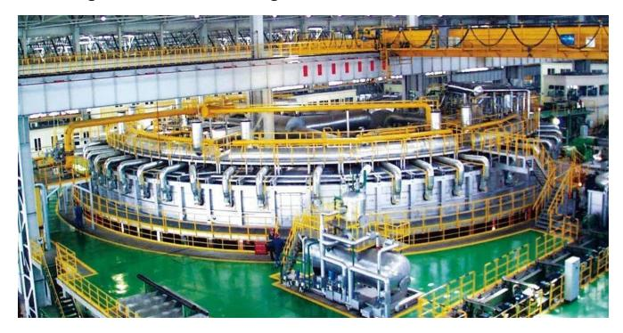
The annular quenching furnace operates continuously, using mixed gas as fuel. Burners are staggeredly arranged on both inner and outer ring walls. The normal furnace temperature ranges from 1000 to 1100°C, with a weakly reductive atmosphere and slightly positive pressure operation.
