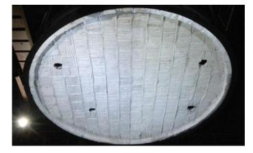
The Steel (Iron) Ladle Preheater generally use gas or oil as fuel to heat the steel (iron) ladle, and the burner is generally located in the center of the dryer. The furnace has a partially reducing atmosphere, the furnace temperature is 800-1000°C, and the temperature that the dryer can bear is about 1000-1200°C.
