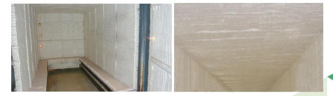
The general requirements for the lining structure of typical vehicle transportation insulation boxes include the following aspects: firstly, they must withstand long-term operation at high temperatures up to 1000°C, have excellent insulation performance, and be resistant to thermal shock. Secondly, they should facilitate
