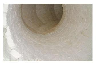
Due to the requirements of various components in the coke oven, ceramic fiber products cannot be applied to the working surface of the oven. However, because of their excellent low volume density and low thermal conductivity, their forms have developed to be functional and complete. The certain
