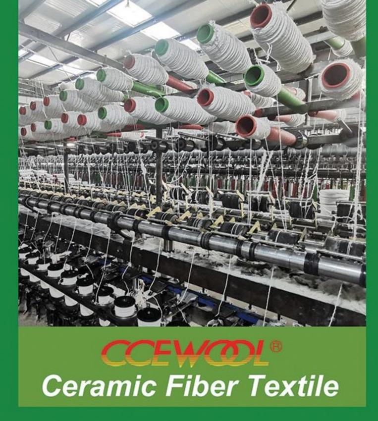
CCEWOOL® ceramic fiber textile includes ceramic fiber yarn, cloth, tape and rope. Using ceramic fiber bulk as raw material and made from ceramic fiber strand, CCEWOOL® ceramic fiber textile offers excellent insulation property.
