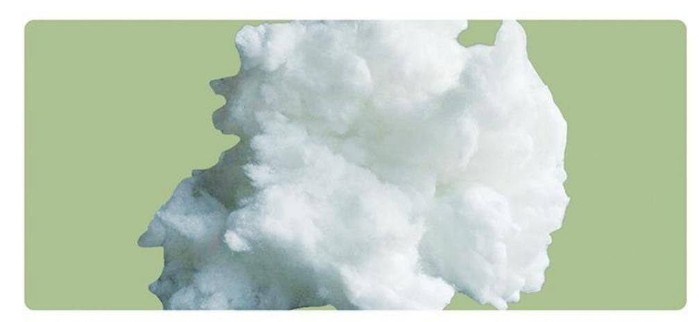
CCEWOOL® Low Biopersistent Fiber Bulk consisits of calcium, magnesium, silicate. The fibers can be degraded in the human body to meet the requirements of health and environmental protection. CCEWOOL® Low Biopersistent Fiber Bulk serves as the foundation for soluble fiber products such as blanket, board.paper and other vacuum-formed products. It can meet European regulatory requirements (Directive 97/69/EC).
