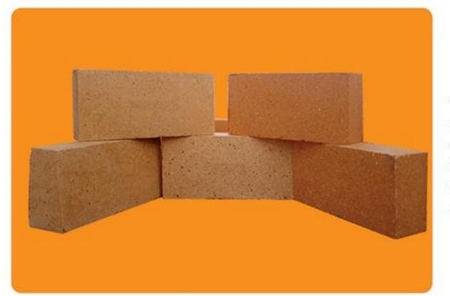
CCEFIRE ® DCHA Series Fire Bricks is the refractory products produced with clay clinker as aggregate and refractory clay as the bonding agent, with Al2O3 content between 30-48%. Fire bricks is the oldest; the most widely used refractory material.
