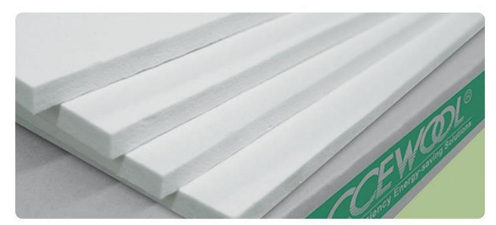
CCEWOOL® Low Biopersistent Fiber Board LT is a soluble fiber board made from a mixture of organic and inorganic binders, with a very low Fe2O3 content. Our CCEWOOL® Low Biopersistent Fiber Board LT can come into direct contact with fire and can be cut into various sizes according to customer requirements. It has an extremely low thermal conductivity, low heat storage capacity, and excellent resistance to thermal shock, making it suitable for applications with large temperature variations.
