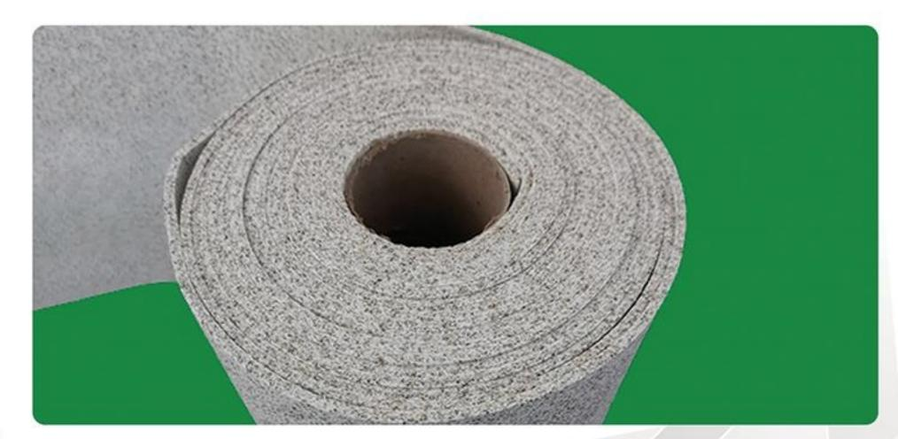
CCEWOOL® Intumescent Ceramic Fiber Paper is produced from a mixture of high purity refractory ceramic fiber, natural graphite fine flakes, and organic binders through a fiber washing process. At about 1200 °F (649 °C), CCEWOOL® Intumescent Ceramic Fiber Paper expands up to maximum of 400% of its thickness. This feature serves as excellent material for gasket and sealing applications.
