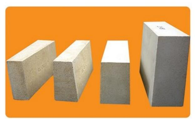
CCEFIRE ® DEHA Series High Alumina Refractory Brick is a kind of neutral refractory material with aluminum content more than 48%. High alumina refractory brick is made through calcination and molding from bauxite and other raw materials with high content of alumina. According to different content of alumina in high alumina brick, its fire resistance, refractoriness under load, compressive strength and other indicators are varied.
