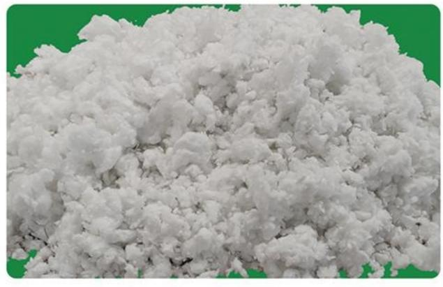
CCEWOOL® Ceramic Fiber Friction Bulk is a combination of refractory ceramic fibers and binding agents, which are designed to improve its characteristics. This type of friction material is manufactured by blending refractory ceramic fibers with organic and inorganic binders. The production process involves mixing, molding, forming, curing, and sintering.
