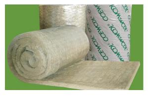
CCEWOOL heat-resistance Rock Wool blanket with Wire Mesh is manufactured in rolls, which is made from rock wool felt and galvanized iron wire mesh or stainless-steel wire mesh sewn together with galvanized iron wire or stainless-steel wire. It features good elasticity, thermal preservation, and easy construction. Water repellent type and low chlorine type of products can be manufactured according to the requirement of customers. Aluminum foil,
