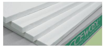
Temperature grade 1200°C (2192°F) CCEWOOL® Low Biopersistent Fiber Board 2192 is a soluble fiber board made from a mixture of organic and inorganic binders, with a very low Fe2O3 content. Our CCEWOOL® Low Biopersistent Fiber boards can come into direct contact with fire and can be cut into various sizes according to customer requirements. It
