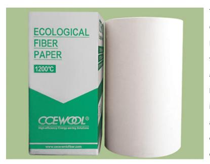
Temperature Grade: 1200°C (2192°F) CCEWOOL® Low Biopersistent Fiber Paper is made from alkaline-earth silicate fibers primarily composed of SiO2, MgO, and CaO, blended with specific organic binders. This soluble fiber product is an innovative solution for high-temperature applications. With its unique calcium-magnesium chemical composition, it meets the requirements of
