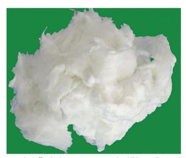
Temperature Grades:  $1100^{\circ}$ C (2012°F),  $1260^{\circ}$ C (2300°F),  $1400^{\circ}$ C (2550°F),  $1430^{\circ}$ C (2600)
