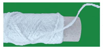
Temperature Grade: 1260°C (2300°F) CCEWOOL® Ceramic Fiber Yarn is made through a special process using refractory ceramic fiber cotton, non-alkali glass filament, and high-temperature-resistant stainless steel alloy wire. It is used for the installation of insulation materials and heat conduction systems and is also widely used in the production of other refractory ceramic
