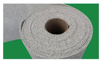
Temperature Grade 1260  $^{\circ}$ C (2300  $^{\circ}$ F) CCEWOOL® Intumescent Ceramic Fiber Paper is produced from a mixture of high purity refractory ceramic fiber, natural graphite fine flakes, and organic binders through a fiber washing process. At about 1200  $^{\circ}$ F (649  $^{\circ}$ C), CCEWOOL® Intumescent Ceramic Fiber Paper expands up to maximum of 400% of its thickness. This feature serves as excellent material for gasket and sealing applications.
