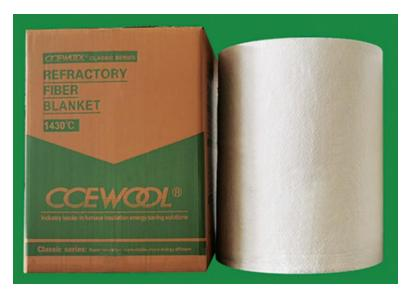
Temperature Grade 1430°C (2600°F) CCEWOOL® Ceramic Fiber Blanket 2600 is made from high-purity alumina, zirconia, and silica as raw materials through a unique fiber manufacturing process. It possesses excellent insulation properties and exhibits extremely low shrinkage characteristics at high temperatures. Its long-term operating temperature reaches around 1350°C (2462°F). This product is white in color, flexible in texture, has good flatness, and is highly temperature-resistant, delivering
