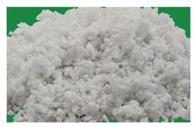
Temperature degree: 1260 °C (2300 °F) CCEWOOL® Ceramic Fiber Friction Bulk is a combination of refractory ceramic fibers and binding agents, which are designed to improve its characteristics. This type of friction material is manufactured by blending refractory ceramic fibers with organic and inorganic binders. The production process involves mixing, molding, forming, curing, and sintering.
