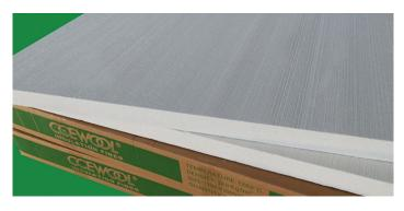
Temperature Grade 1400 °C (2550 °F) CCEWOOL® Ceramic Fiber Board LZ is a zirconium alumina refractory ceramic fiber board made from low-zirconium refractory ceramic fiber spun cotton as raw material, produced through a fully automated vacuum forming process. It operates continuously for 24 hours and dries quickly, resulting in better compressive strength. The surface is smooth, the dimensions are
