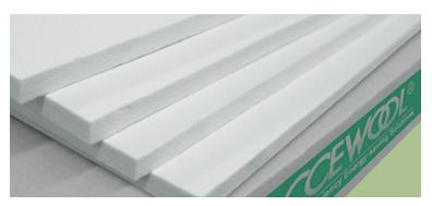
Temperature grade 1200 °C (2192°F) CCEWOOL® Low Biopersistent Fiber Board 2192 is a soluble fiber board made from a mixture of organic and inorganic binders, with a very low Fe2O3 content. Our CCEWOOL® Low Biopersistent Fiber boards can come into direct contact with fire and can be cut into various sizes according to customer requirements. It
